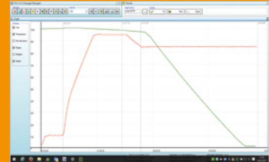
Simultaneous display of temperature (red) and loss in weight (green)
