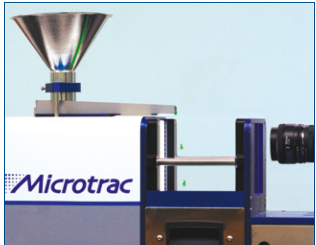
Key elements of PartAn 3D system
