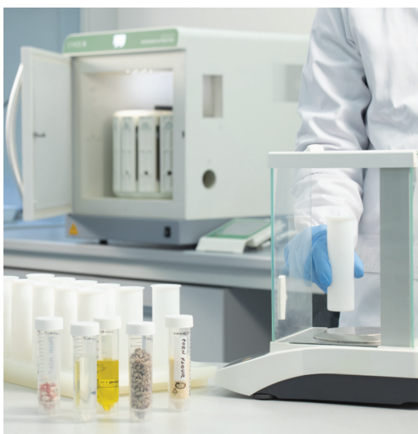
1 - Weighing step on the hydrolysis/ extraction vessel
