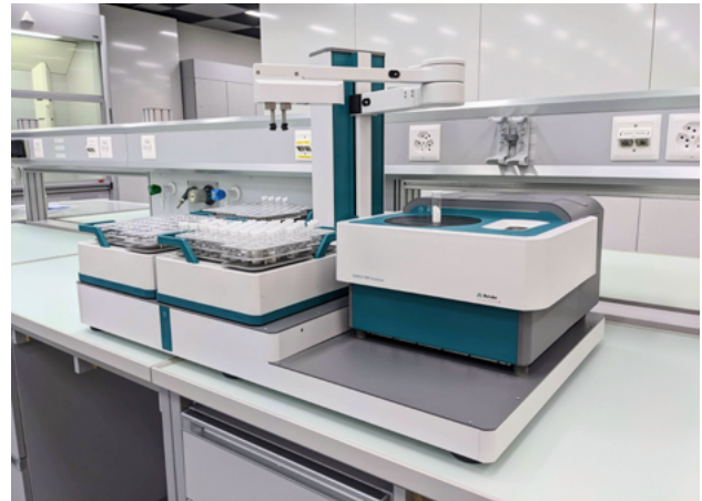
Figure 13. OMNIS Sample Robot – NIR with different racks for different vial sizes. One sample vial is positioned for measurement on the OMNIS NIR Analyzer and is automatically exchanged by the sample robot arm once analyzed.
