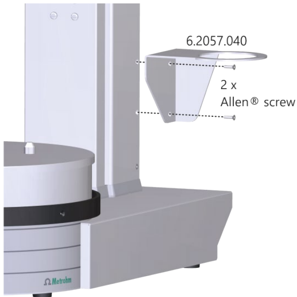
Figure 3. Mounting the holder for Dosino on the 858 Professional Sample Processor.
