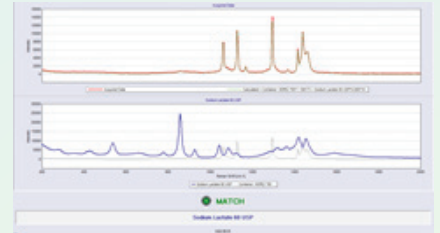
Figure 7. Identification result of sodium lactate 60% in thick HDPE2 container
