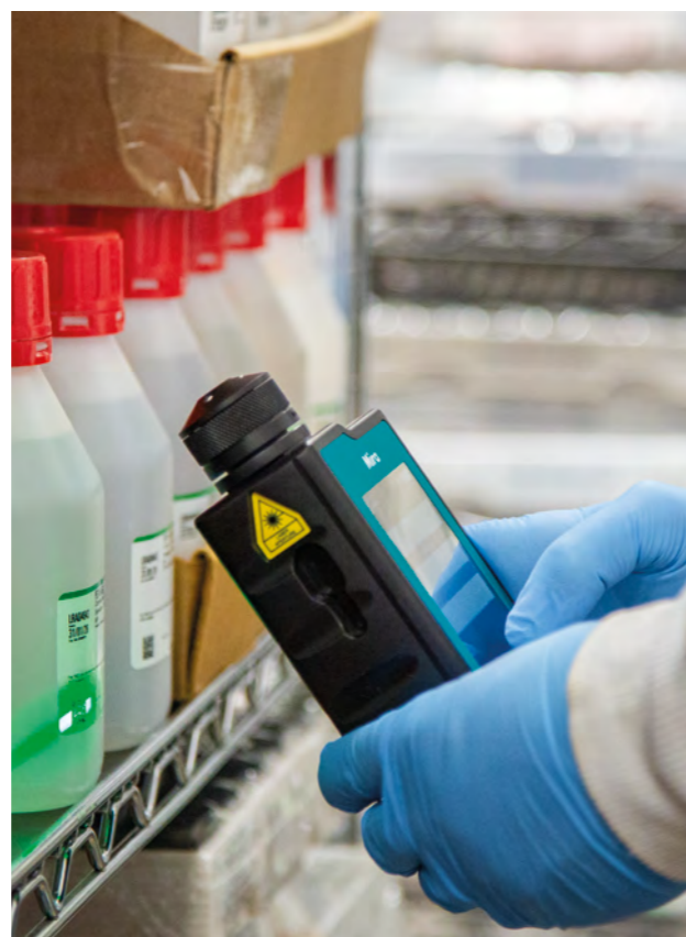
The integrated barcode scanner supports the capability of MIRA P to quickly test 100% of a batch.
