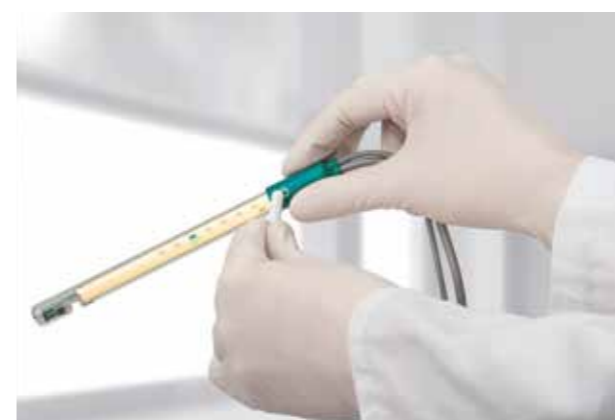
b) Simply touch the magnet symbol on the head of the electrode with the supplied magnetic stirring bar ...
