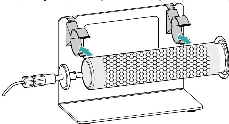
4. Place the adsorption cartridge holder with the CO<sub>2</sub> adsorption cartridge CW into the instrument's detector chamber.
