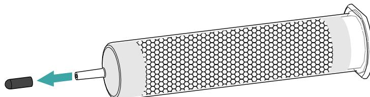
2. Attach the dust filter to the tip of the CO<sub>2</sub> adsorption cartridge CW.
