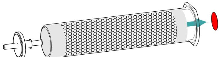
This uncovers the small opening in the lid of the CO<sub>2</sub> adsorption cartridge CW, through which air is aspirated.
