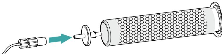
3. Clamp the CO<sub>2</sub> adsorption cartridge CW in place using the clips on the adsorption cartridge holder.
