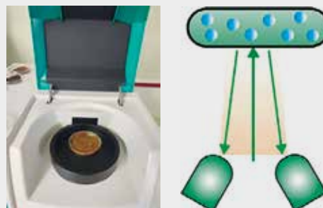
Figure 3 Stool sample with DS2500 Solid Analyzer and the measuring mode diffuse reflectance.
