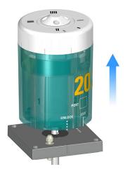
• Raise the cylinder unit OMNIS special straight upwards.
