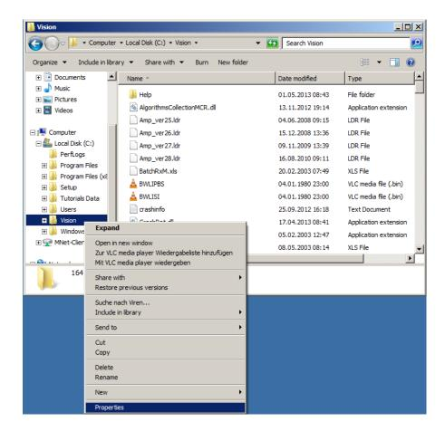
4 In Properties dialog select Tab Security. If the tab is not available, it means you do not have sufficient rights in Windows. You can not run Vision software.
