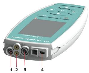
Figure 4 914 pH/Conductometer (analog) - connectors
