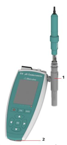
Figure 6 912/913/914 Meter for mobile application
