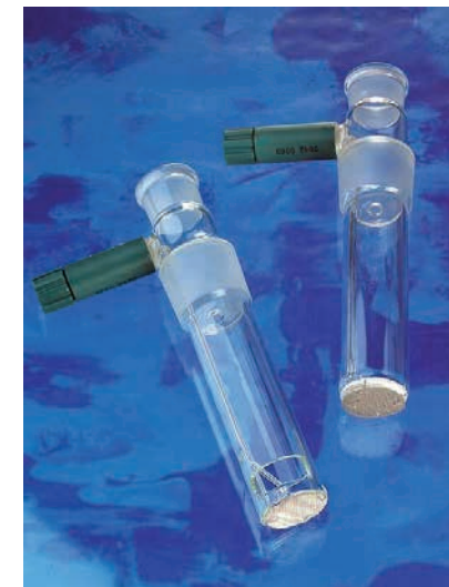
Generator cells for Metrohm KF Coulometers: on the left without, on the right with diaphragm
