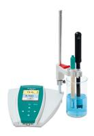
**Figure 1.** 914 pH/DO/Conductometer equipped with an O2-Lumitrode and conductivity sensor for the determination of dissolved oxygen in wine samples.
