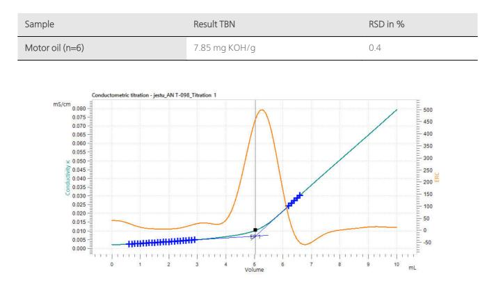
Figure 2. Example titration curve to determine the total base number in motor oil according to IP test method 400.
