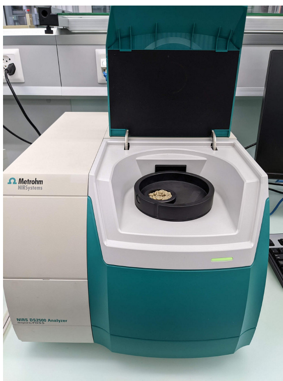
Figure 1. A Metrohm DS2500 Solid Analyzer with green coffee beans held in a NIRS mini sample cup.
