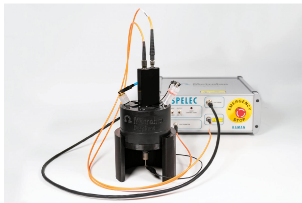
Figure 1. SPELEC RAMAN instrument and Raman probe used in combination with a Raman spectroelectrochemical cell for conventional electrodes.
