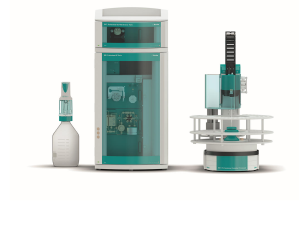
Figure 1. Instrumental setup including a 940 Professional IC Vario (center), 947 Professional UV/VIS Detector Vario SW (top center), 858 Professional Sample Processor (right), and MiPCT-ME, performed with the Metrosep A PCC 2 HC/4.0 and a Dosino (left).
