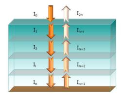
Figure 2. Normal reflection configuration.
