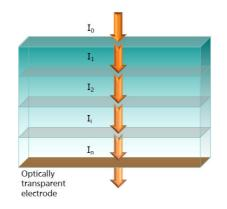
Figure 1. Normal transmission configuration.
