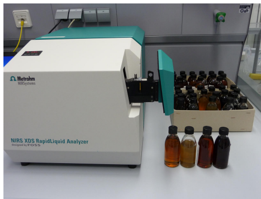
Figure 1. XDS RapidLiquid Analyzer and lubricant samples.
