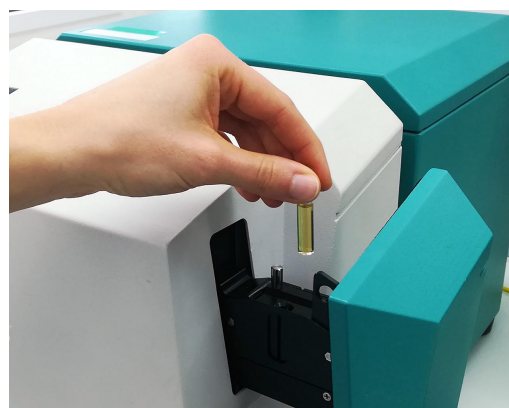
Figure 1. XDS RapidLiquid Analyzer and an isocyanate sample present in the 8 mm Disposable Vial.
