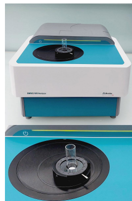
Figure 1. OMNIS NIR Analyzer Solid with 15 mm vial and Flexible holder OMNIS NIR.
