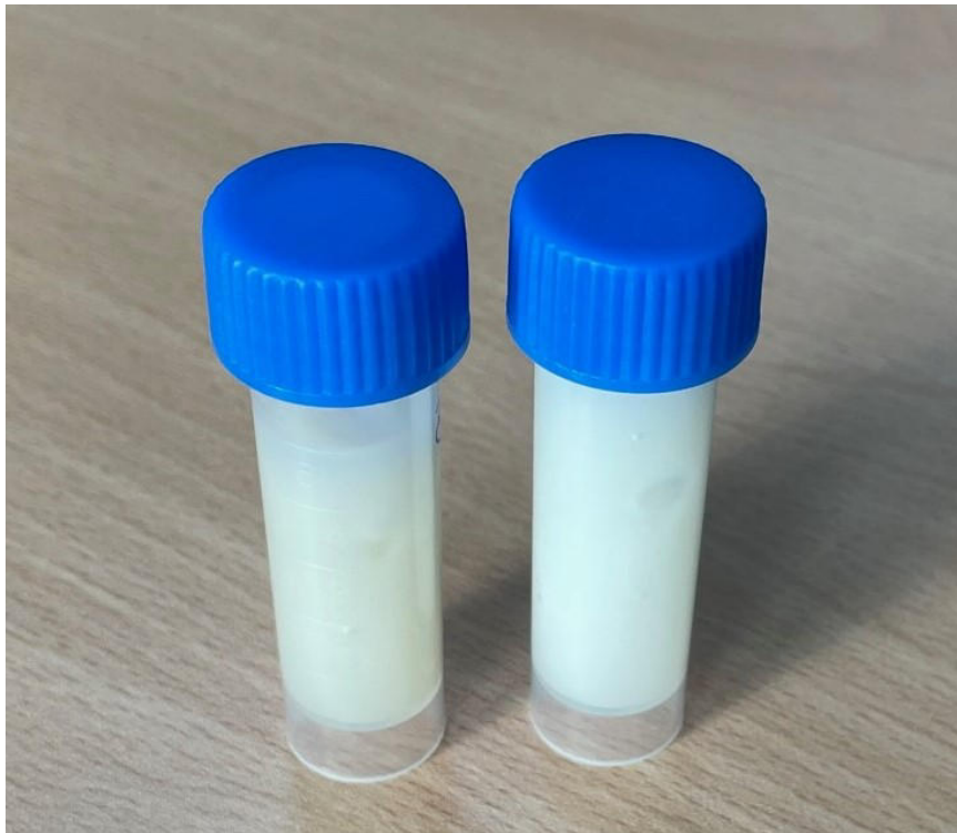
Figure 2. Cold-extracted fat from ground sausages. The petroleum ether was removed at 15 mbar at room temperature.
