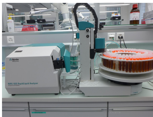
Figure 1. XDS RapidLiquid Analyzer with 5.0 mm flow cell and the 815 Sample Processor.
