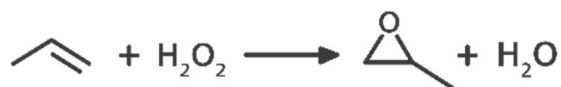
Reaction 1. Overall reaction for the epoxidation of propylene with hydrogen peroxide (HP-PO).
