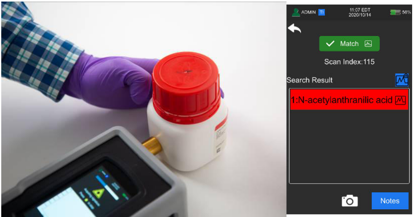
Figure 4. TacticID-1064 ST measurement through HDPE bottle and match result for N-acetylanthranilic acid
