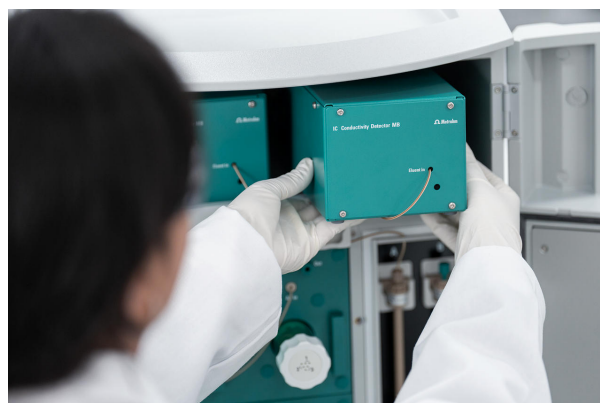
Figure 1. The IC Conductivity Detector MB shown here has a reduced cell volume and is inert against methanesulfonic acid.
