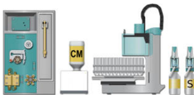
Figure 1. Setup for drinking water testing using a 930 Compact IC Flex with automatic KOH eluent generation (948 Continuous IC Module, CEP), an 858 Professional Sample Processor, and the Metrohm intelligent Partial-Loop Injection Technique (MiPT).
