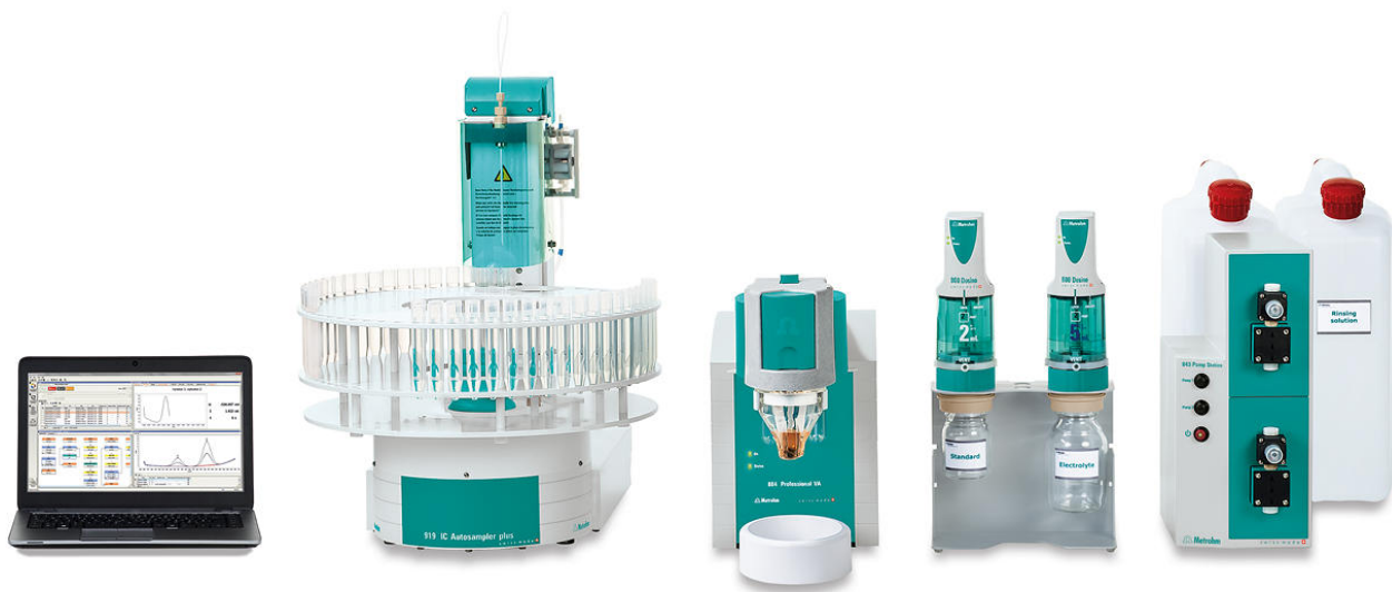
Figure 1. 884 Professional VA, fully automated for VA analysis
