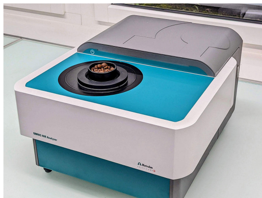
Figure 1. OMNIS NIR Analyzer Solid with roasted coffee beans in the small cup OMNIS NIR, 60 mm.
