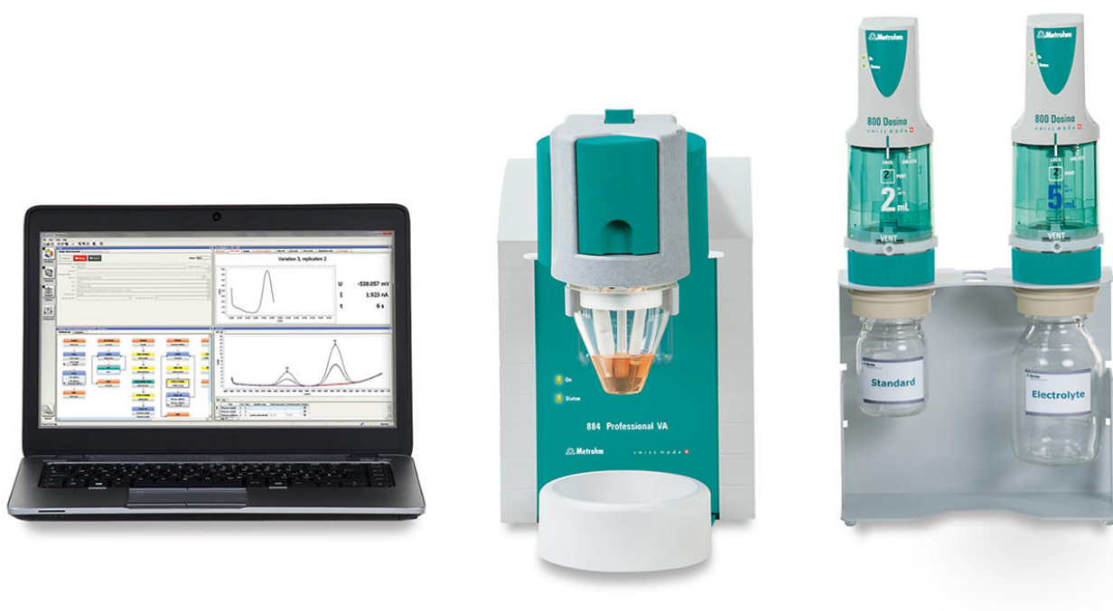
Figure 2. 884 Professional VA, semiautomated for VA analysis
