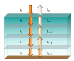
Figure 2. Normal reflection configuration.
