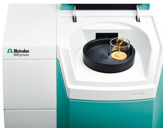
Figure 1. Metrohm DS2500 Solid Analyzer with a NIRS transfection vessel shown instead of a mini sample cup.
