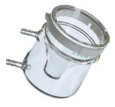
6.1418.220 Titration vessel with thermostat jacket / 20-90 mL
