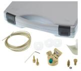
Equipment comprised of Wall-Jet cell with additional accessories. For cyanide analysis with a silver working electrode and a Pd reference electrode.
