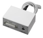
807 Dosing Unit with integrated data chip with 50 mL glass cylinder and light protection, mountable to a reagent bottle with ISO/DIN GL 45 glass thread. FEP tubing connection, antidiffusion tip.
