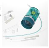
807 Dosing Unit with integrated data chip with 50 mL glass cylinder and light protection, mountable to a reagent bottle with ISO/DIN GL 45 glass thread. FEP tubing connection, antidiffusion tip.
