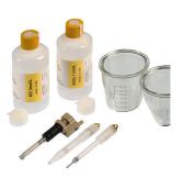
Complete electrode set for the determination of organic additives in electroplating baths with CVS (Cyclic Voltammetric Stripping). Contains rotating platinum working electrode (electrode diameter: 2 mm), driving axle with mercury contact, maintenance-free gel reference electrode, platinum auxiliary electrode, measuring vessels and KCl electrolyte solution.
