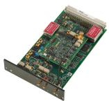
The pX1000 module can also be used as an additional differential electrometer, with the same specifications as the main Autolab electrometer. The pX1000 module is compatible with the Metrohm pH and temperature sensors.
