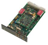
The pX1000 allows the measurements of pH or pX values during electrochemical experiments. This module also provides an additional Pt1000 input which allows recording of the temperature during the experiments, either through a Pt1000 sensor or through a combined pH /Pt1000 sensor. The temperature measurement allows automatic pH corrections.
