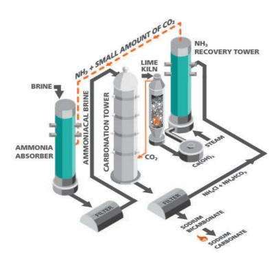
Figure 1. Illustration of the Solvay process used to manufacture sodium carbonate when mining for ore is not economically feasible.
