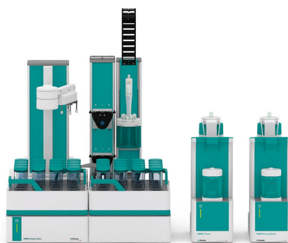
Figure 1. Sample Robot S with Dis-Cover functionality, Dosing module, and OMNIS Advanced Titrator equipped with dPt Titrode for the determination of peroxide value in edible oils.
