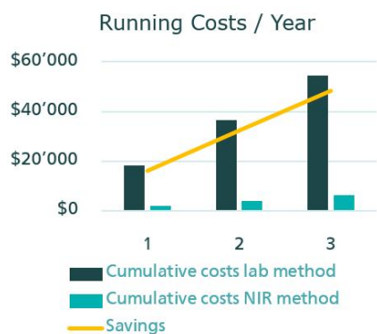
Figure 4. Comparison of the cumulative costs over three years for the determination of the hydroxyl number with titration and NIR spectroscopy.
