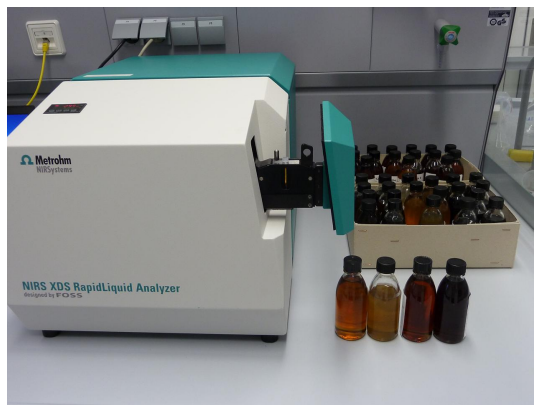
Figure 1. XDS RapidLiquid Analyzer and lubricant samples.
