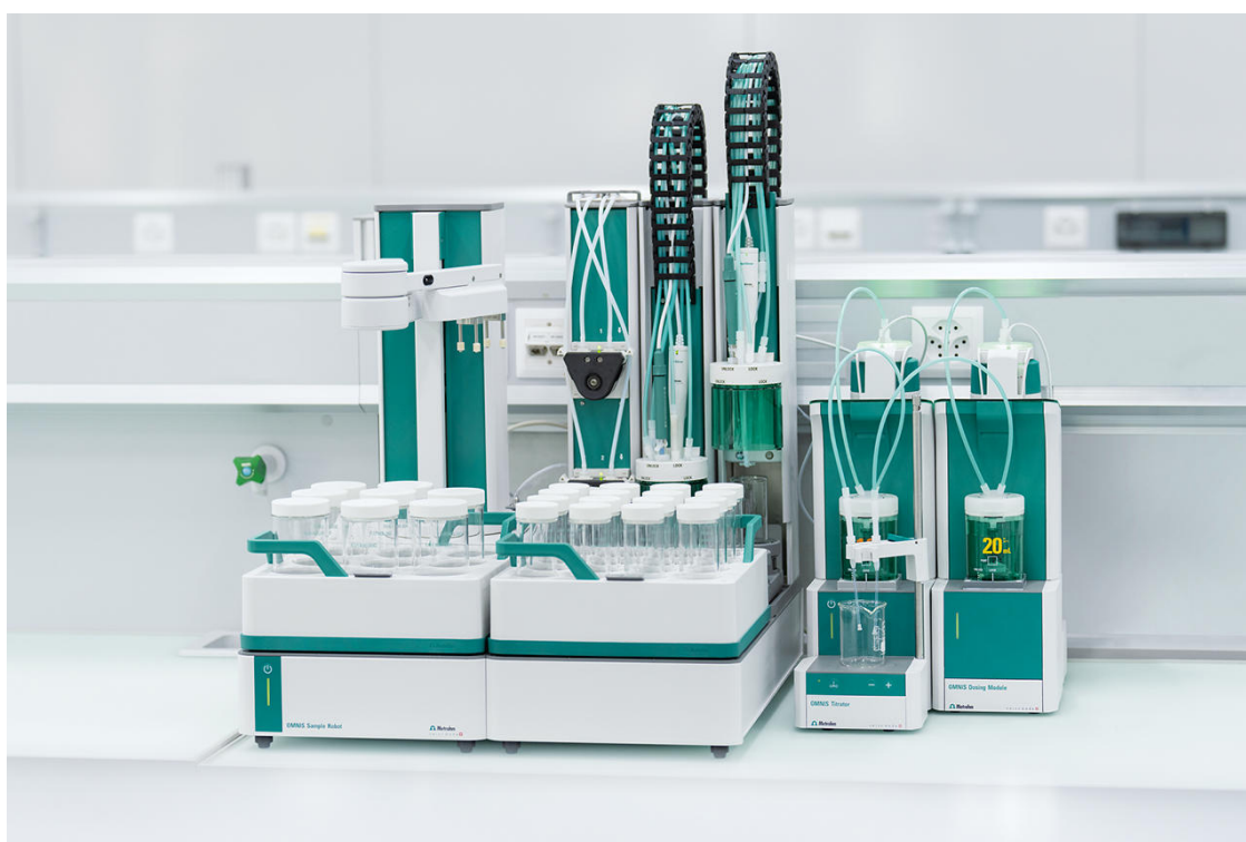
Figure 1. OMNIS Sample Robot S equipped with an OMNIS Titrator, Dosing module, and dUnitrode electrode for the automated determination of pyrophosphate in aqueous samples.
