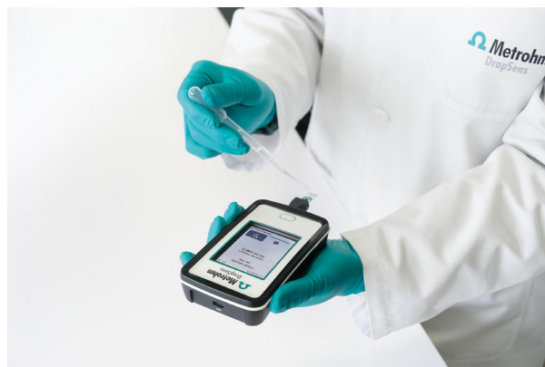
Figure 5. Example of a novel handheld setup where a miniaturized ion-selective screen-printed electrode is utilized with a portable potentiostat to make on-site measurements.
