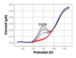
Figure 2. Determination of chromium(VI) in tap water spiked with 30  $\mu\text{g/L}$
