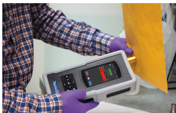
Figure 1. TacticID-1064 ST measuring a sample through a manila envelope with ST adapter
